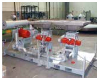
Two different raw material loading at the same time with the Double Chamber Silo Loading Unit SYRB
