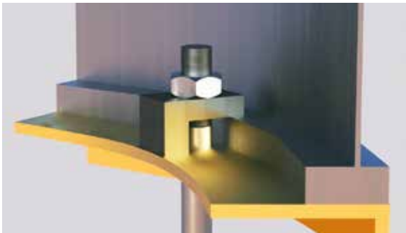
Silo Anchor Assembly
